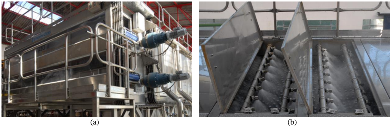
Figure 1. (a) Tunnel Pasteurizer and (b) bottles being heated by water sprays inside the tunnel.
