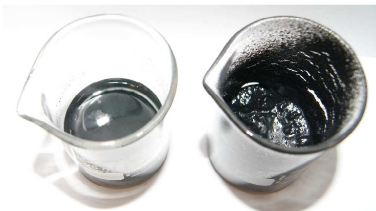
Figure 9. Beaker containing the nanofluid dispersion. The left side before the sonication process and right side after sonication process.
