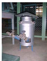
Figure (8) Pico-hydro generator Source: (Tiago Filho and Duarte, 2006).
