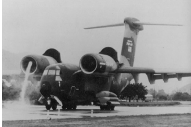
Fig. 1 Ground vortex on an YC-14 aircraft (Campbell and Chambers, 1999)
