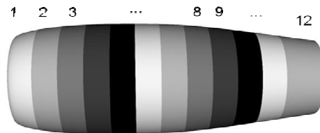
Figure 10 – Nacelle with splitted external walls.
