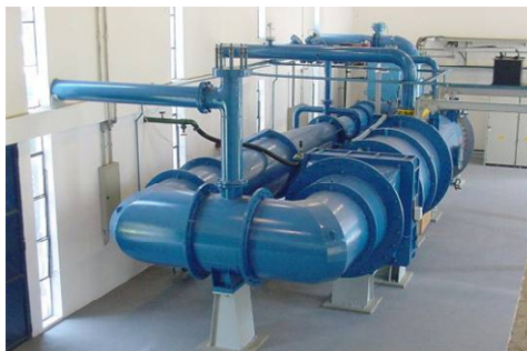
Figure 1. Aerodynamic circuit and the operational envelope of PTT.
