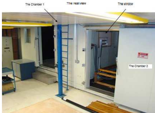
Figure 3. Calorimeter apparatus containing two chambers.
