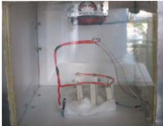
Figure 2. Resistive assembly for the thermal load variation
