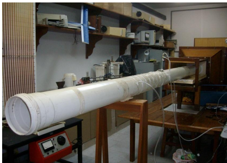
Figure 1. PVC pipe connected to the wind tunnel
