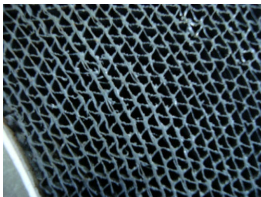
Figure 2. Micro channels of the desiccant rotor.
