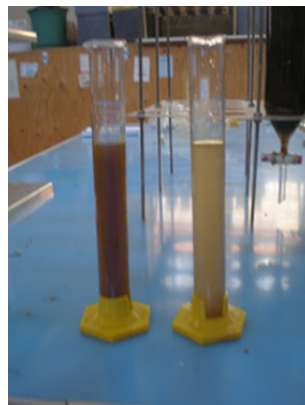
Figure 5. Water(80%)/oil(20%) mixtures collected after flowing through a globe (right) and a cyclonic (left) valve.
