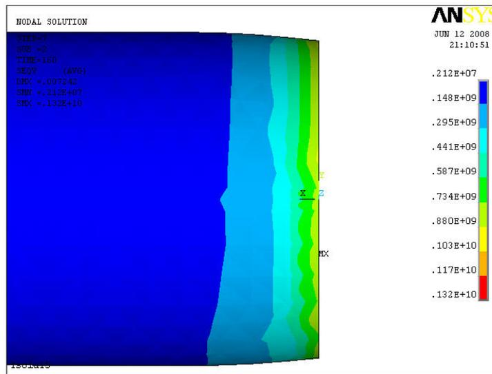
Figure 7 Detail of von Mises stresses at position D
