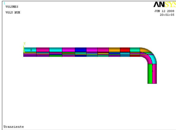
Figure 6 ANSYS model of the pipe experimental section
