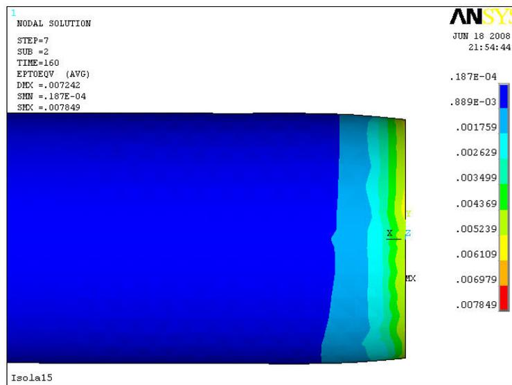
Figure 8 Detail of von Mises strains at position D
