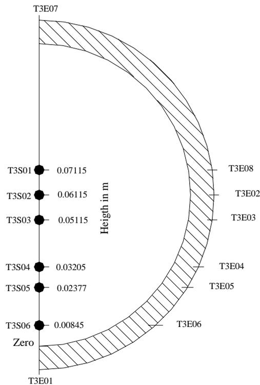
Figure 5 Inside and outside thermocouples of measuring position III
