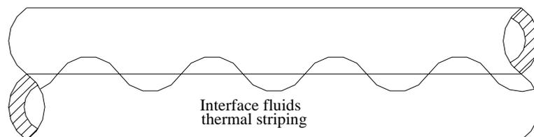
Figure 3 Thermal striping in the fluids interface
