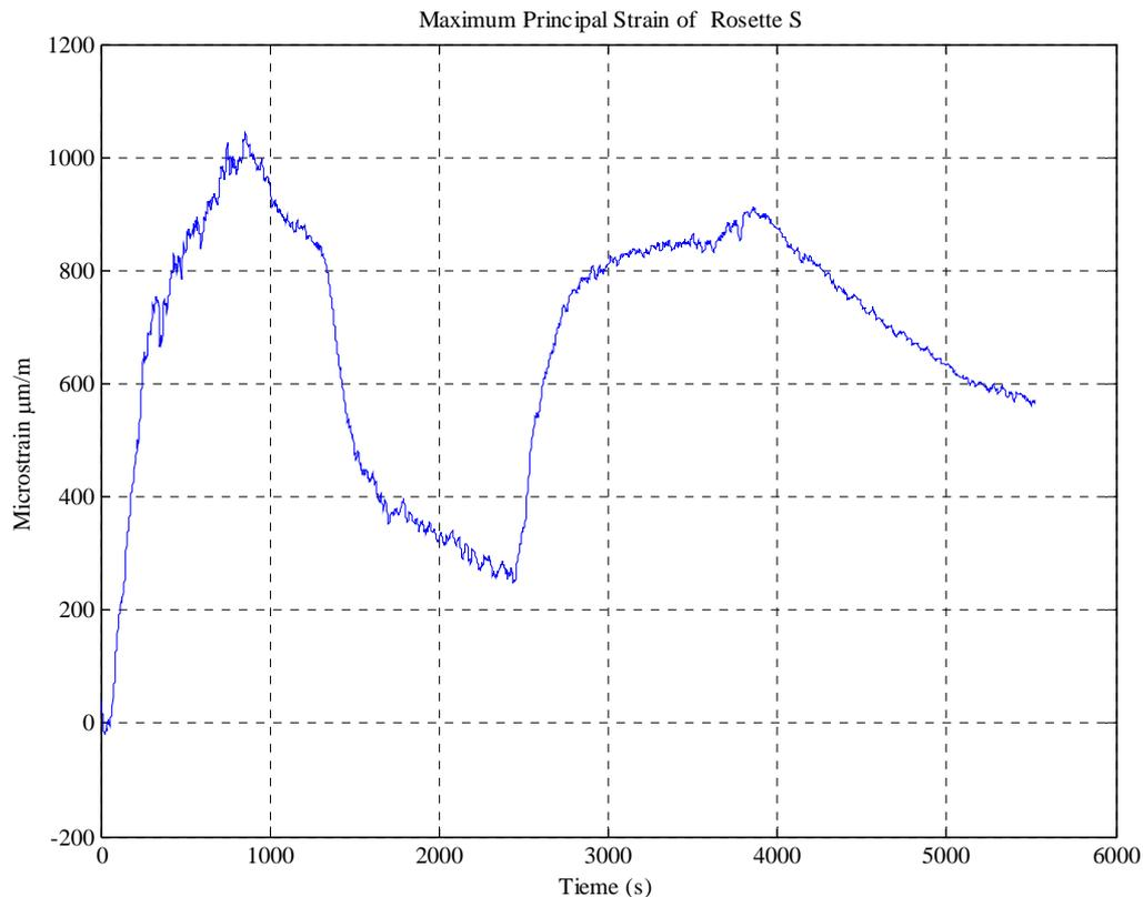
Figure 11 Strains measured at position D
