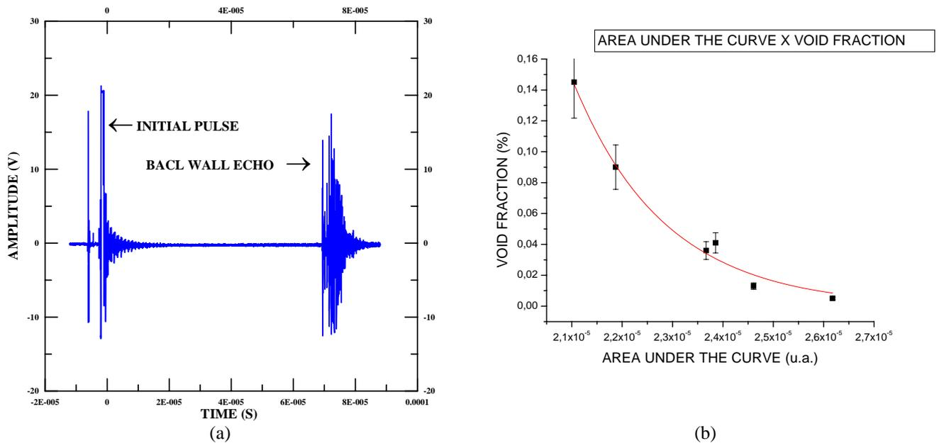
Figure 4. (a) Typical echogram and (b) Void fraction as a function of the area under the back wall echo curve.
