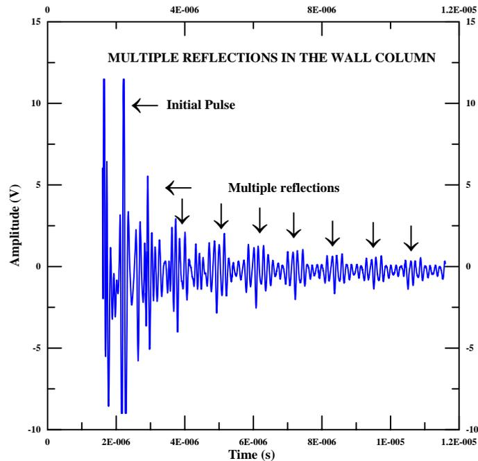
Figure 3. Multiple Reflections in the wall glass column.
