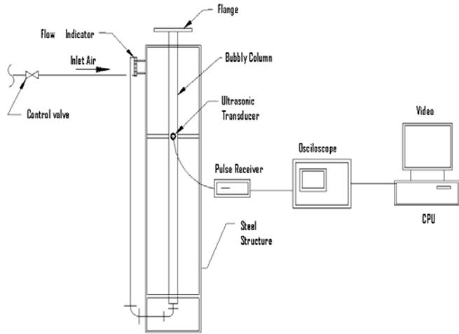
Figure 1. Schematic of the experimental facility.
