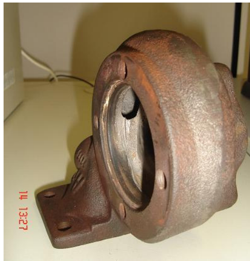
Figure 2: Box of Spiral Turbo-Compressor used as a model for the measurement
