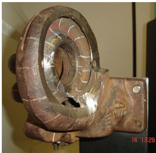
Figure 4: Box Spiral of Turbo - Compressor with the internal boundaries for the measurement
