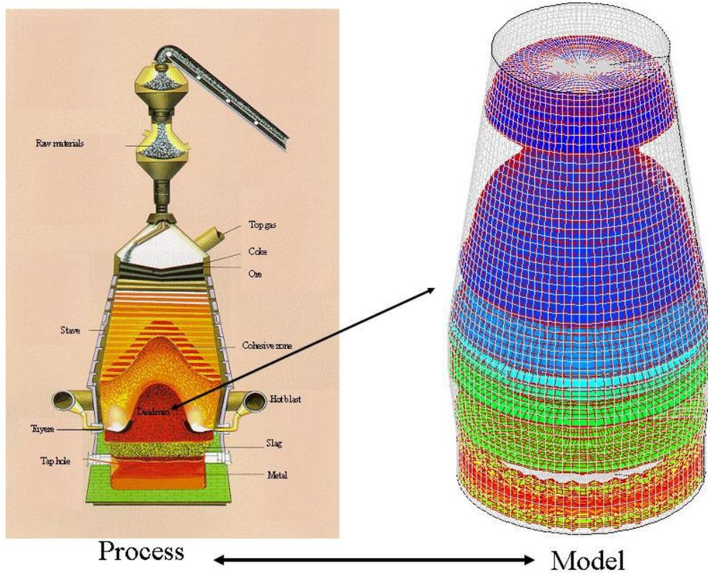
Figure 1 Inner zones and finite volume mesh generated to simulate the compact blast furnace process
