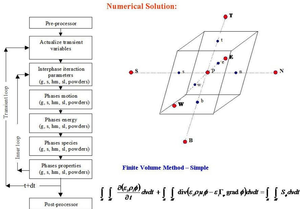
Figure 3 algorithm and computational molecule for the mini blast furnace model
