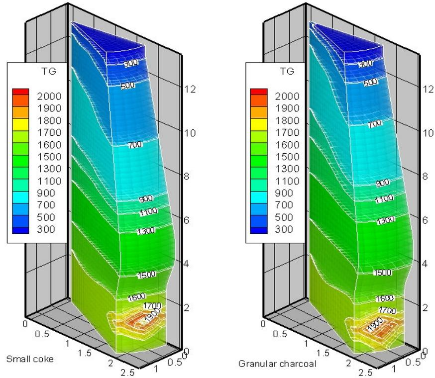
Figure 4 comparison of gas phase inner temperature distribution for mini blast furnace operation based on small coke and charcoal
