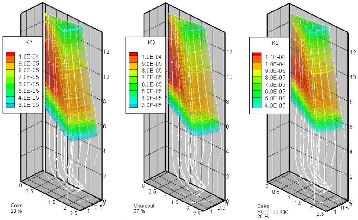
Figure 7 Potassium circulation in the furnace burden for high utilization of self-reducing agglomerates
