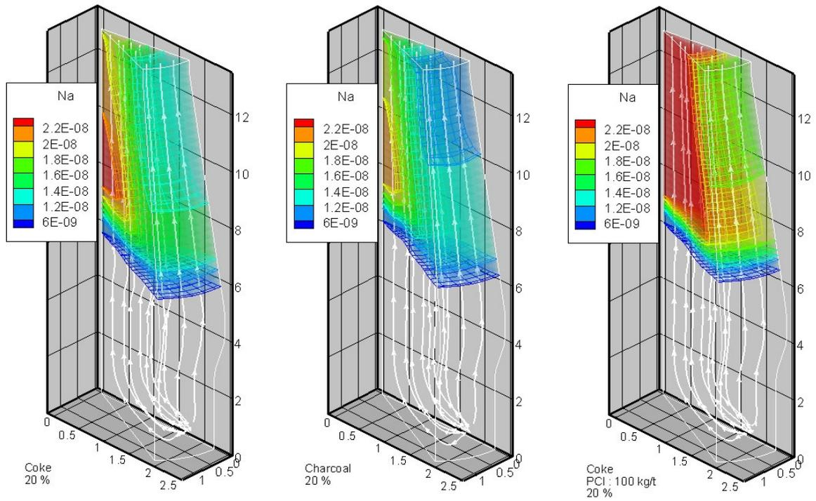
Figure 6 Comparison sodium recirculation and gas flow pattern with high amount of self-reducing agglomerates for both coke and charcoal based operations
