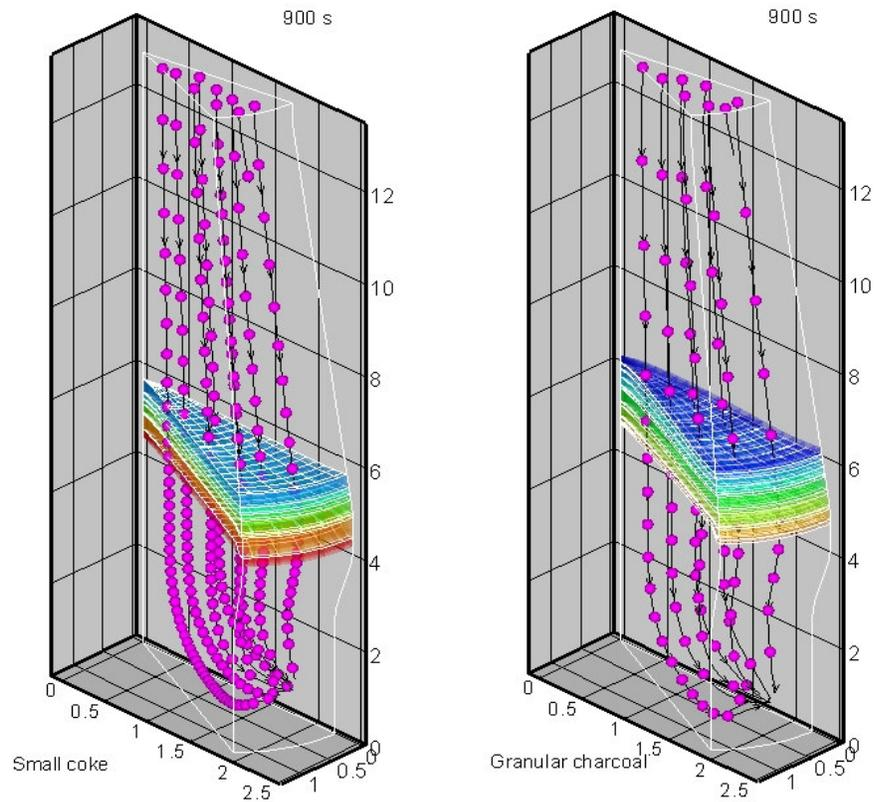
Figure 5 Comparison of solids motion and cohesive zone location for mini blast furnace operation based on small coke and charcoal
