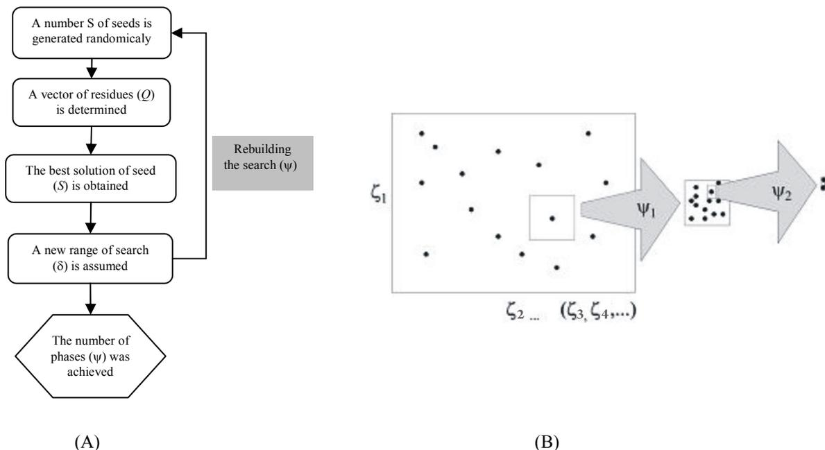
Figure 1. Flowchart of the R2W algorithm (A) with the schematic representation (B)
