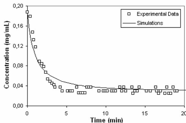
Figure 4. Correlation between the R2W inverse method (lines) and the experimental adsorption data (points) of the insulin on Accel Plus QMA<sup>®</sup>. Where  $C_{A0} = 0,188 \text{ mg/mL}$
