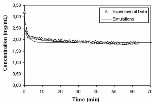
Figure 6. Correlation between the R2W inverse method (lines) and the experimental adsorption data (points) of the insulin onto Accel Plus QMA<sup>®</sup>. Where  $C_{A0} = 3,211$  mg/mL
