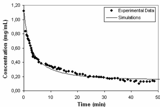
Figure 5. Correlation between the R2W inverse method (lines) and the experimental adsorption data (points) of the insulin onto Accel Plus QMA<sup>®</sup>. Where  $C_{A0} = 1,120$  mg/mL
