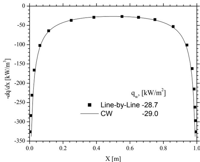
Figure 2 - Radiative source and net wall flux for water vapor medium at 1000 K.
