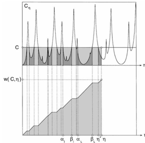
Figure 1 – Cumulative wavenumber function (Solovjov and Webb, 2002).
