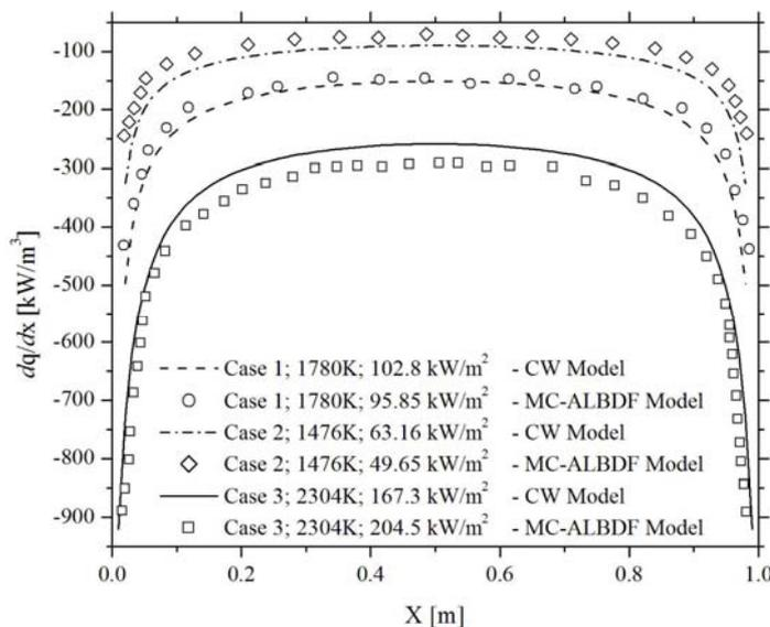
Figure 4 – Comparison to the results obtained from CW model in the present work and MC-ALDF model (Maurente, 2006b).
