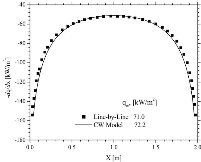
Figure 3 - Radiative source and net wall flux for a gas medium with 20 % water vapor at 1500 K.
