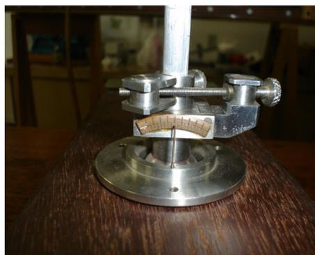
Figure 3. Mechanism of angle variation.
