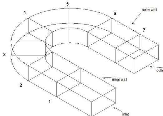
Figure 5 – Schematic draw of the seven planes on the curved channel.
