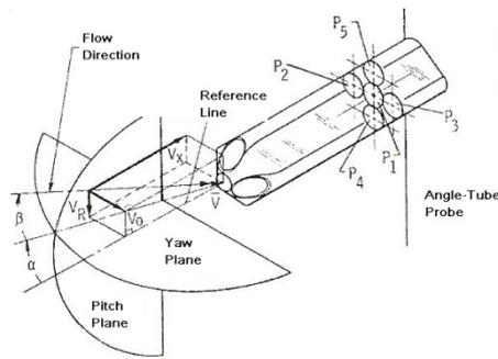
Figure 4. The pressure probe
