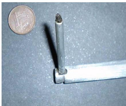
Figure 2. The five-holes pressure probe.
