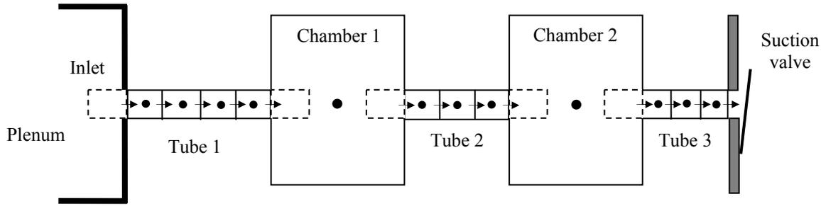
Figure 1. Staggered finite volume grid arrangement adopted in the finite volume methodology.
