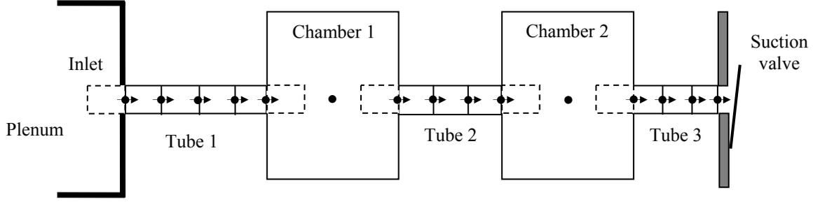
Figure 2. Non-staggered grid arrangement adopted in the finite difference methodology.
