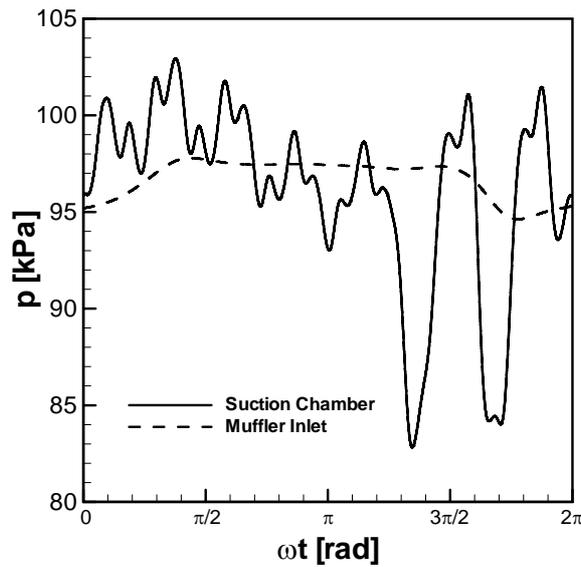
Figure 4. Pressure attenuation in the muffler.
