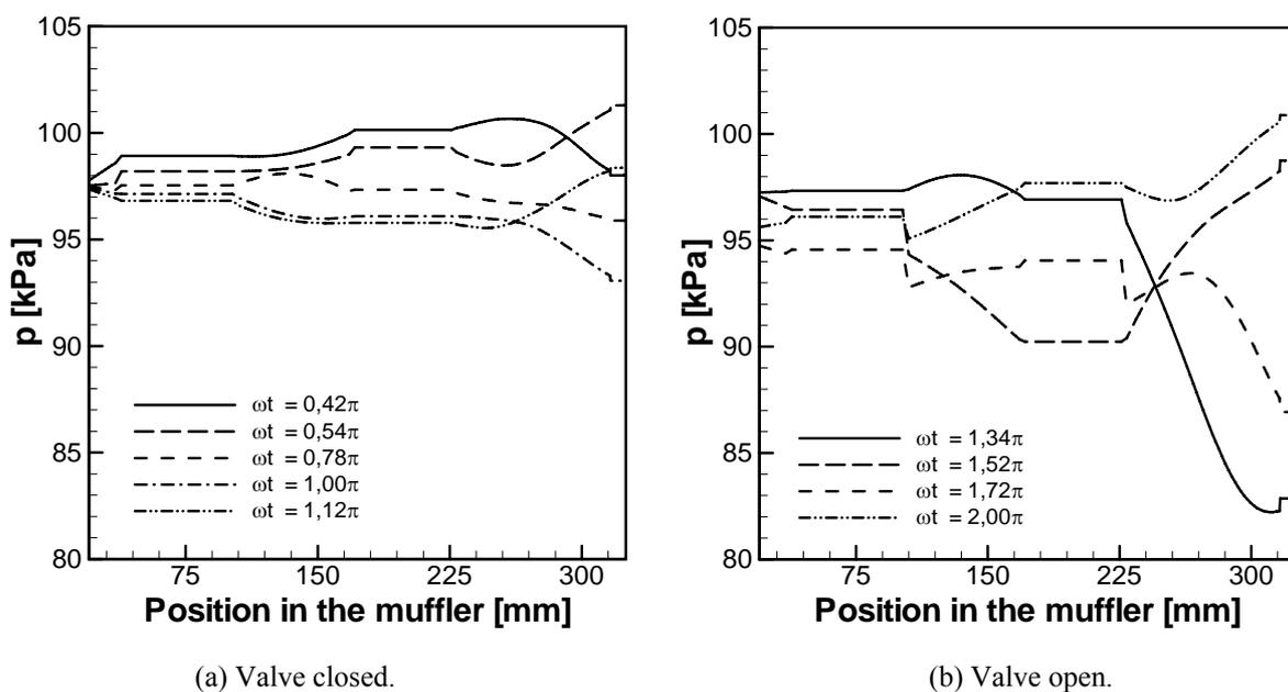
Figure 5. Pressure distribution along the muffler length.
