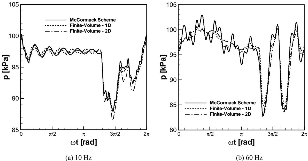
Figure 3. Results for pressure pulsation in the suction chamber.
