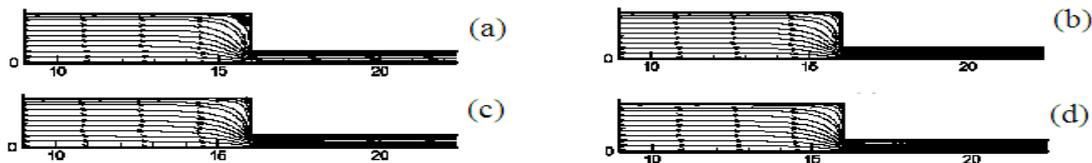
Figure 5: A detail of flow streamlines at the sudden contraction region for  $n=2$  and  $Re=2$ : (a)  $Cu=0$ , (b)  $Cu=10$ , (c)  $Cu=50$  and (d)  $Cu=100$ .
