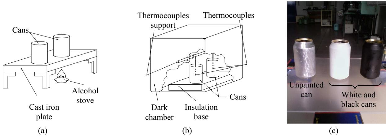
Figure 3: Experimental devices: (a) water and cans heating system; (b) dark chamber of tests; (c) metallic cans of tests.
