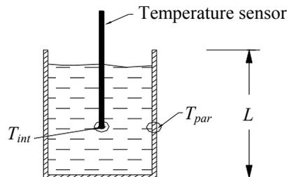
Figure 2 – Can filled with water ( $T_{int} > T_{par}$ ).
