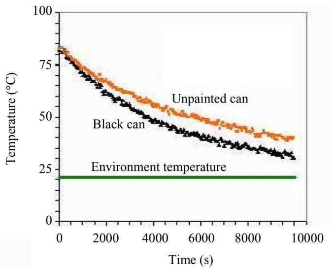
Figure 5: Comparison between the unpainted can and the can painted in black.
