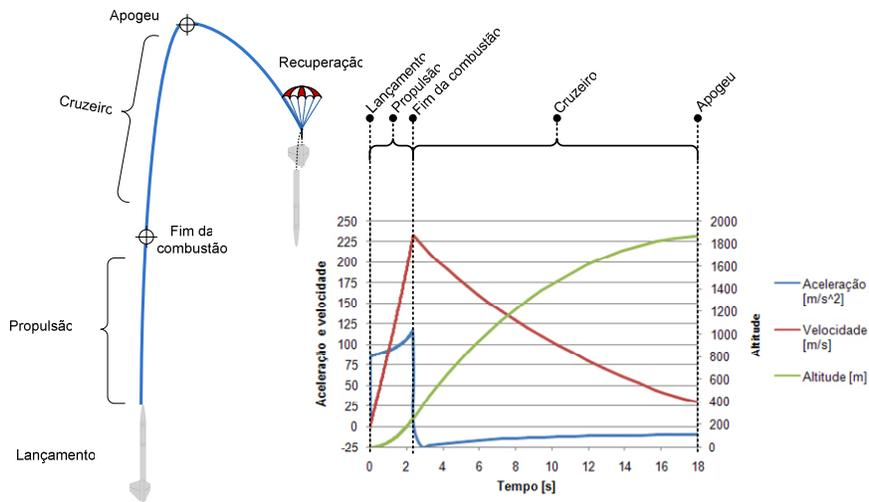
Figure 9. Free flight rocket main events and the relation with acceleration, speed and altitude.
