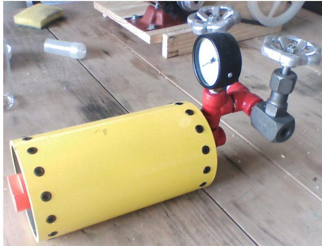
Figure 2. An equipment for solid propellant characterization, developed by the author, and presented on the website (Porto, 2007).
