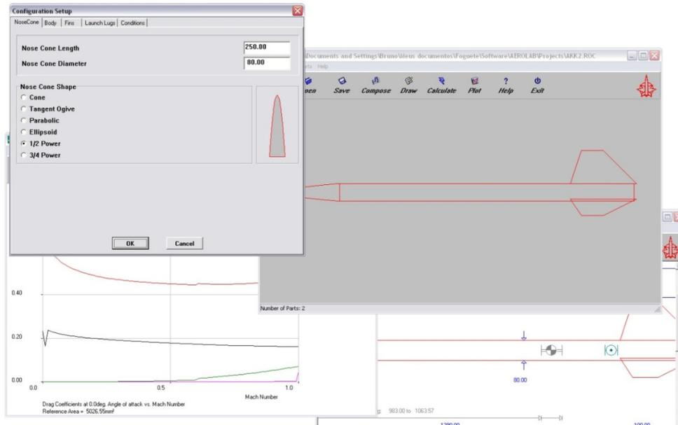
Figure 4. Aerolab software for stability and drag calculation (Nakka, 2007).
