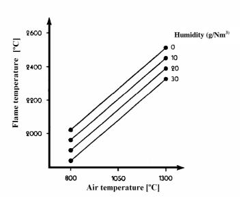
Figure 2. Effect of air temperature on the combustion flame temperature
