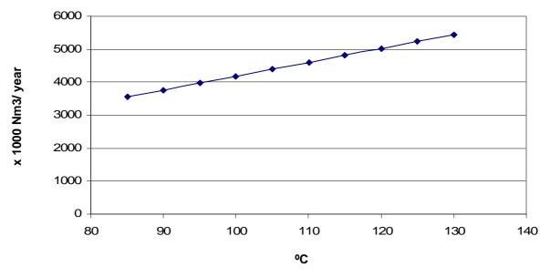
Figure 6. Annual saving of oxygen as a function of air temperature increase
