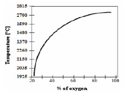
Figure 1. Effect of the oxygen concentration on the combustion flame temperature
