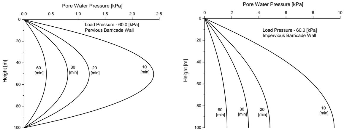
Figure 5 – Height versus Pore water pressure for different times (Porous barricade wall) and pervious barricade wall (left plot) and impervious barricade wall (right plot)
