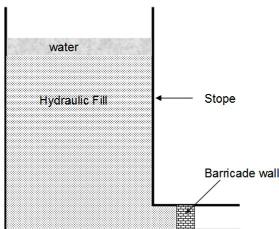
Figure 1 - Typical hydraulic fill stopes
