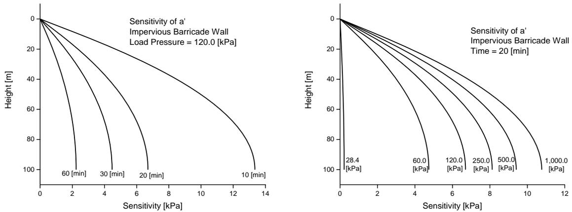
Figure 7 – Sensitivity of Coefficients  $a$  and  $\xi$  with respect to time and position (height) (left) and with respect to load pressure and position (height) (right)
