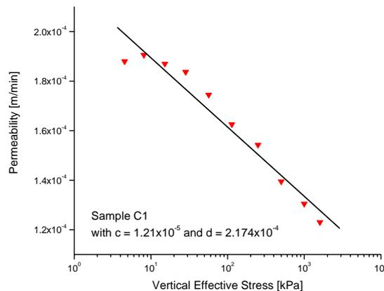
Figure 3 – Permeability versus Vertical effective stress (right), adapted from Singh *et al.* (2008).
