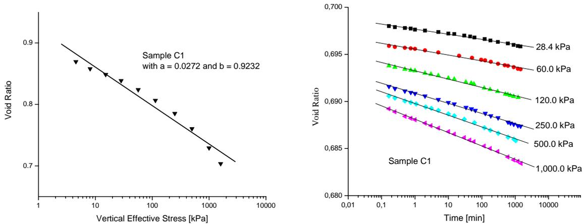
Figure 2 – For sample C1, void ratio versus vertical effective stress (left), adapted from Singh *et al.* (2008), and void ratio versus time (right), adapted from Singh and Sivakugan (2008).
