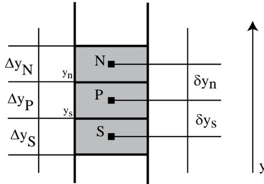
Figure 4 – Schematic diagram of the control volume used to integrate Eq. (9).
