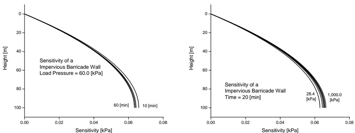
Figure 6 – Sensitivity of Coefficients  $a$  and  $\xi$  with respect to time and position (height) (left) and with respect to load pressure and position (height) (right)
