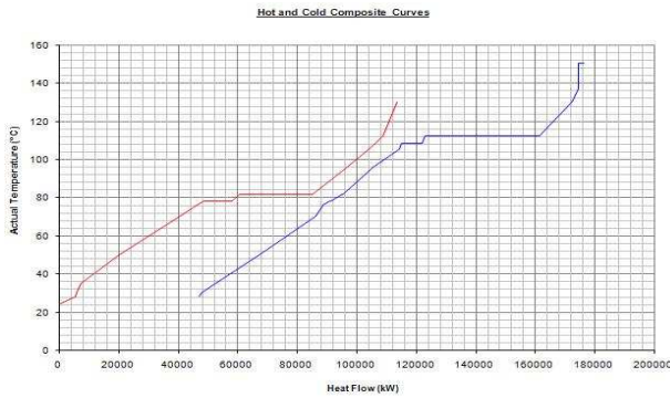
Figure 7. Composite Curves for conventional distillation case.
