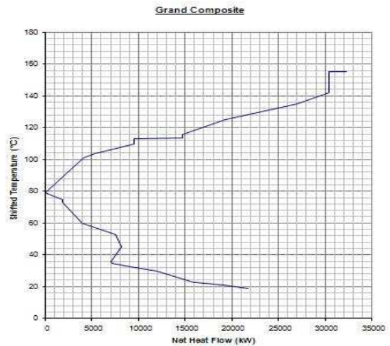
Figure 10. Grand Composite Curves for the double-effect distillation case.
