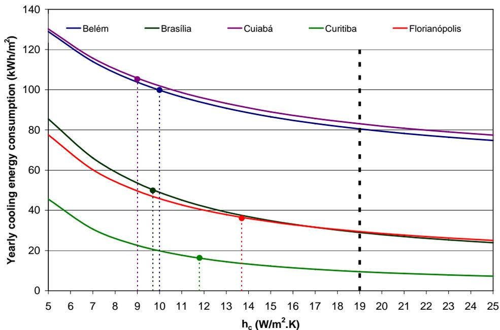
Figure 3. Yearly cooling energy consumption as a function of the external CHTC imposed value.
