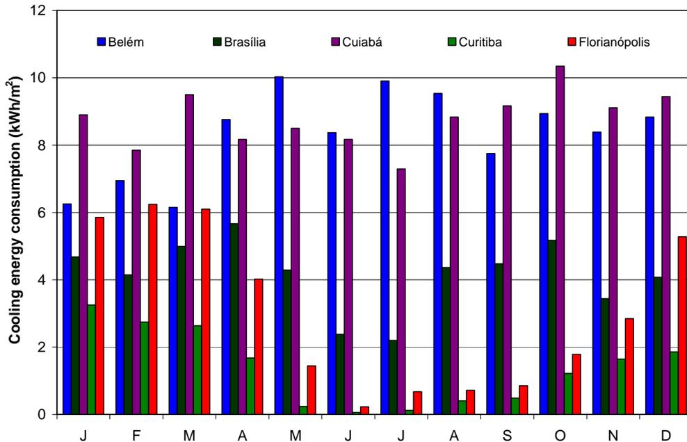
Figure 2. Monthly cooling energy consumption.
