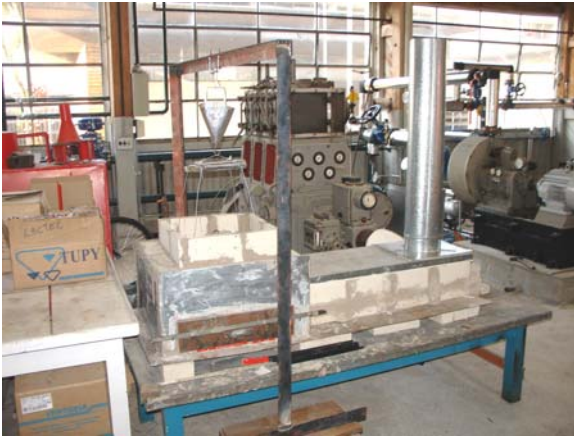
Figure 5. Natural draft furnace with no external insulation
