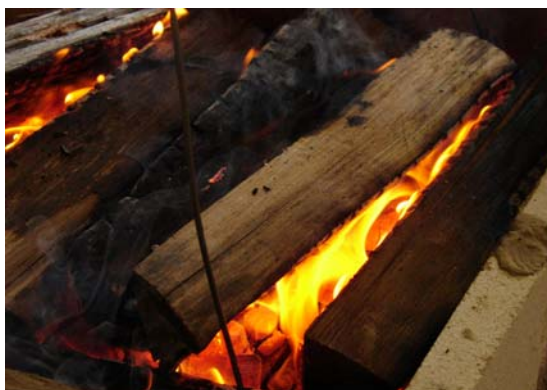
Figure 8 . Illustration of flame showing the concurrent flow.
