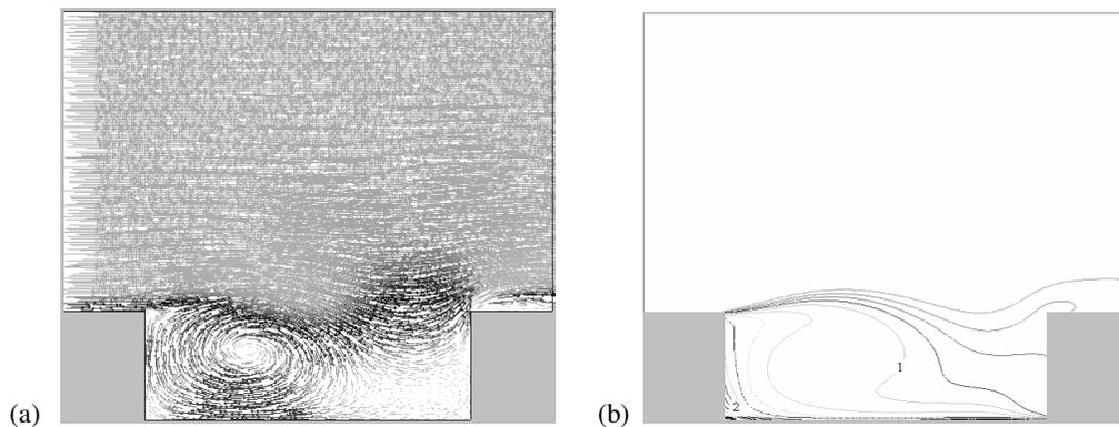
Figure 2. Wind field (a) and concentration distribution (b) for an aspect ratio of 0.333
