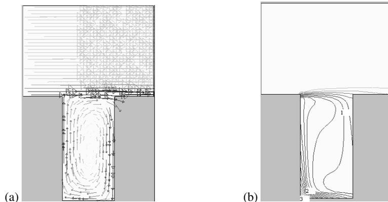
Figure 5. Wind field (a) and concentration distribution (b) in a street canyon with aspect ratio of 2.0 for leeward side heating
