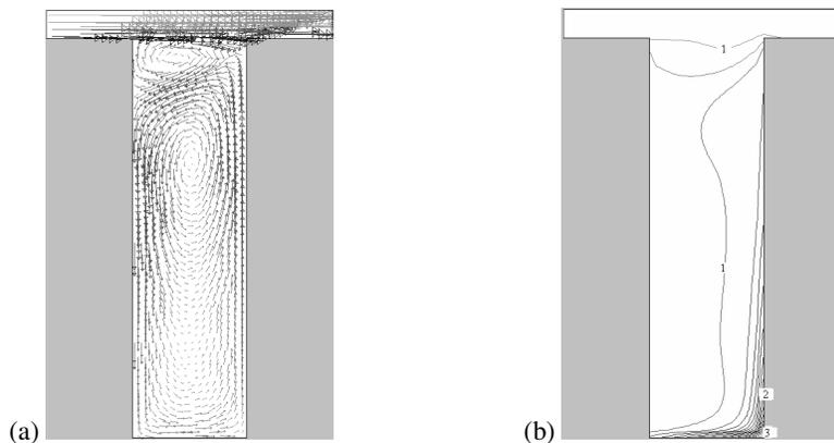
Figure 6. Wind field (a) and concentration distribution (b) in a street canyon with aspect ratio of 3.5 for windward side heating
