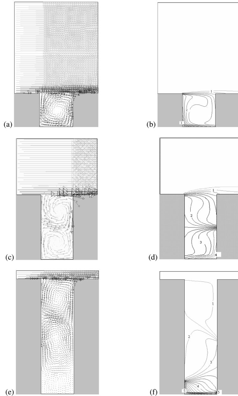
Figure 3. Wind field and concentration distribution in street canyons with aspect ratios of 1 [(a) and (b)], 2 [(c) and (d)], and 3.5 [(e) and (f)]
