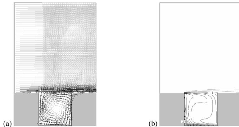
Figure 4. Wind field (a) and concentration distribution (b) in a street canyon with aspect ratio of 1.0 for bottom heating
