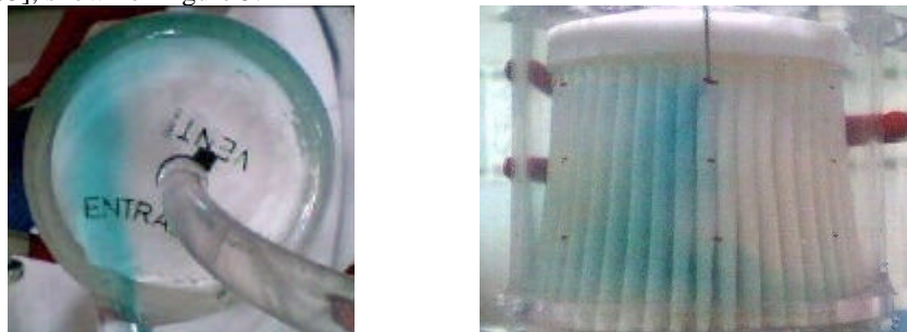
Figure 5. Top view showing the flow direction and the division at the exit connector neighborhood (Huebner, 2003)
