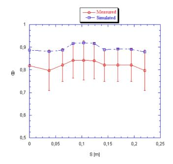
Figure 5. Comparison between calculated and measured temperature for normal blood flow
