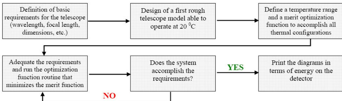
Figure 6 – Flow diagram for optimization, Leite Jr and Silva (2007)
