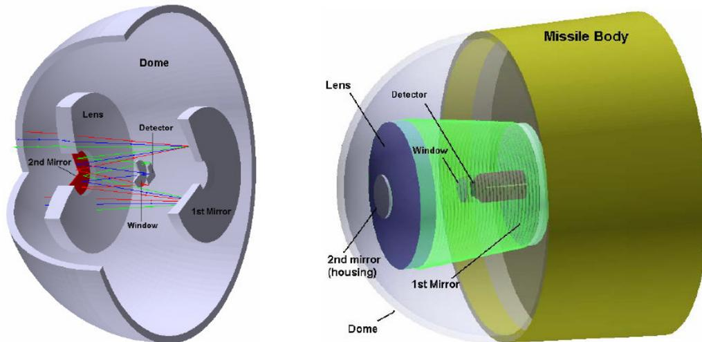
Figure 1 – Optical system proposed
