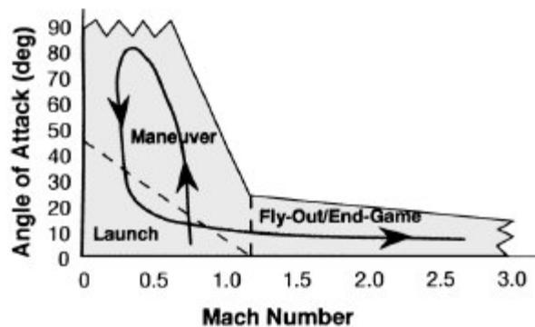
Figure 3 – Agile missile flight envelope (Wise and Roy, 1998)
