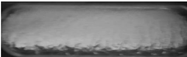
(e) R-407C with \omega=3.0\% , G=200 \text{ kg/s.m}^2 , vapor quality =91% and h = 319 \text{ W/m}^2.\text{K} .
