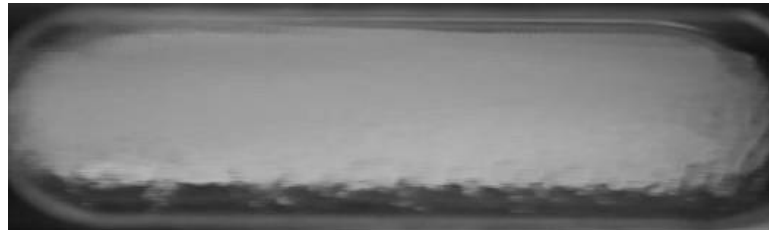
(b) R-407C with \omega=1.0\% , G=200 \text{ kg/s.m}^2 , vapor quality =94% and h=185 \text{ W/m}^2.\text{K} .
