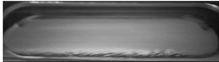
(a) Pure R-407C with G = 100 \text{ kg/s.m}^2 , vapor quality=76% and h = 915 \text{ W/m}^2.\text{K} .
