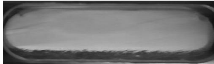
(b) R-407C with \omega=0.5\% G = 100 \text{ kg/s.m}^2 , vapor quality=70% and h = 1229 \text{ W/m}^2.\text{K} .
