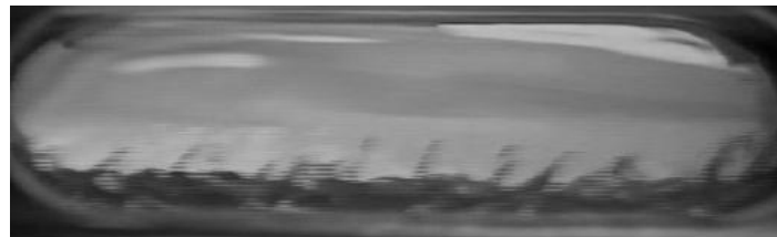
(d) R-407C with \omega=5.0\% , G = 100 \text{ kg/s.m}^2 , vapor quality=80% and h = 85 \text{ W/m}^2.\text{K} .
