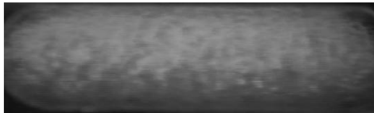
(c) R-407C with \omega=3.0\% , G=200 \text{ kg/s.m}^2 , vapor quality =84% and h = 2178 \text{ W/m}^2.\text{K} .
