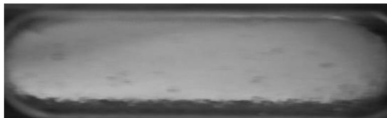
(d) R-407C with \omega=3.0\% , G=200 \text{ kg/s.m}^2 , vapor quality =84% and h = 2178 \text{ W/m}^2.\text{K} .
