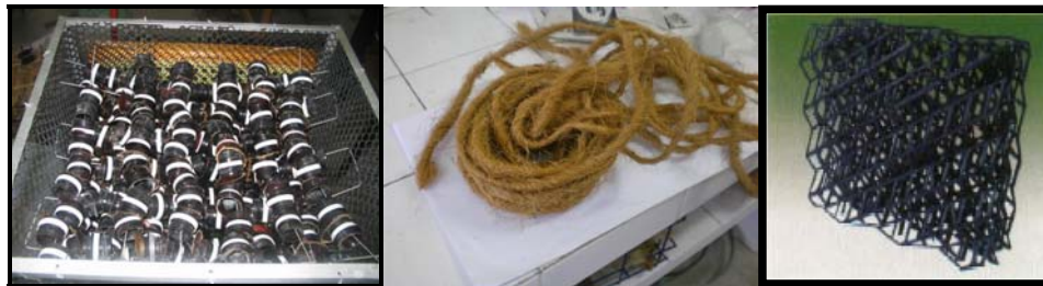
Figure 1. P.E.T. (PET) and coconut fiber (FDC) acting as packing for a cooling tower. They were tested against a commercial cooling pad (INDUSTRIAL).
