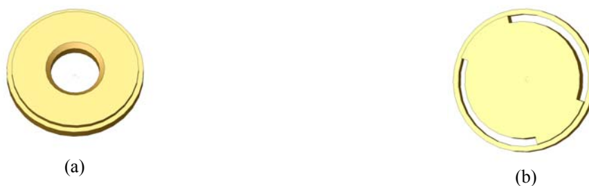
Figure 2. Schematics of outlet orifices: (a) cold orifice (82.81 mm 2 ), and (b) hot orifice (78.54 mm 2 ).
