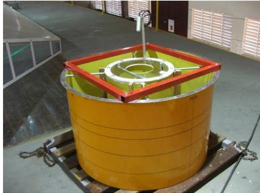
Figure 1. The aluminum monocolumn model – scale 1:100.
