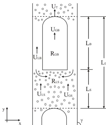
Figure 1. Vertical slug flow unit.
