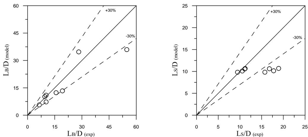
Figure 4. Bubble and slug dimensionless lengths.
