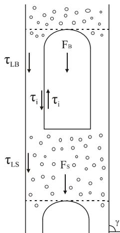
Figure 3. Gravitational forces and shear stresses in the unit cell.
