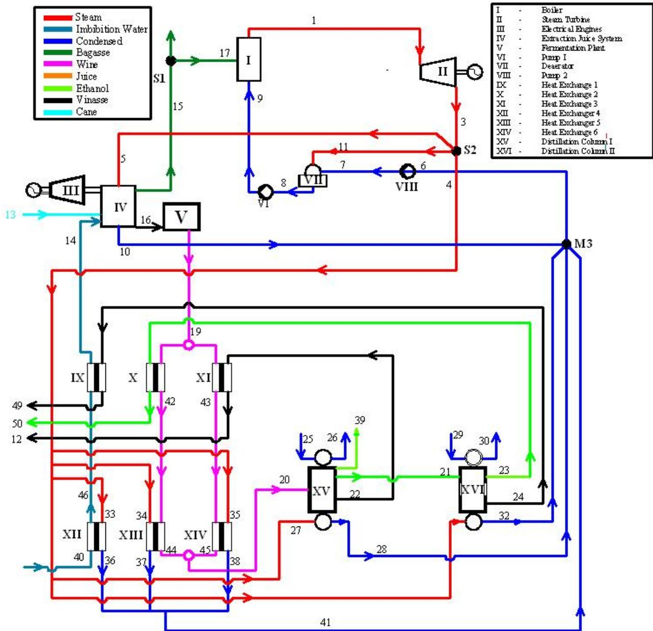
Figure 2 Sketch to cogeneration system integrated with extraction and distillation system through pinch technology
