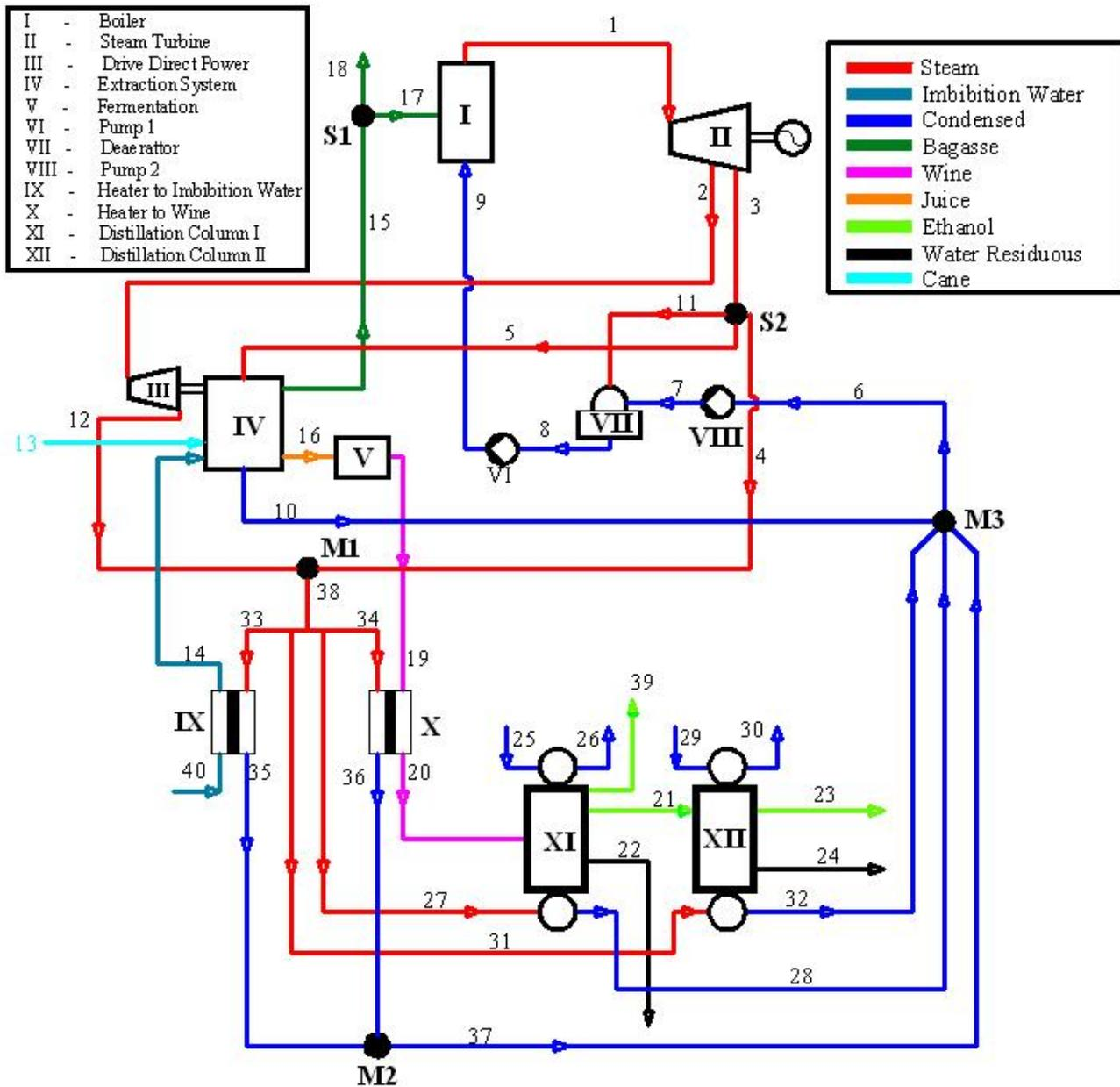
Figure 1 Sketch of Cogeneration, Extraction and Distillation Systems
