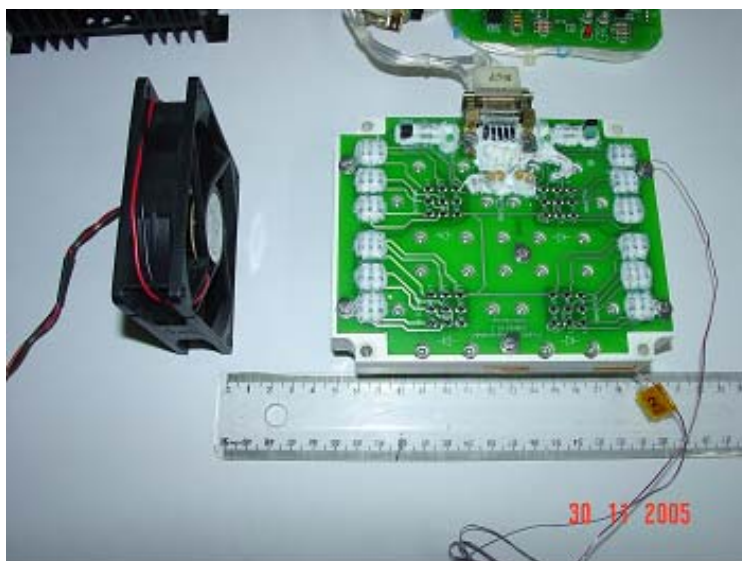
Figure 2. Evaluation of the fan cooling efficiency for the IM main block.
