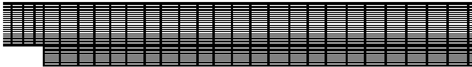
Figure 4 – Slice of the computational domain of the backward facing step discretized in 13 by 51 (entrance) and 121 by 81 (tunnel span) grid points.
