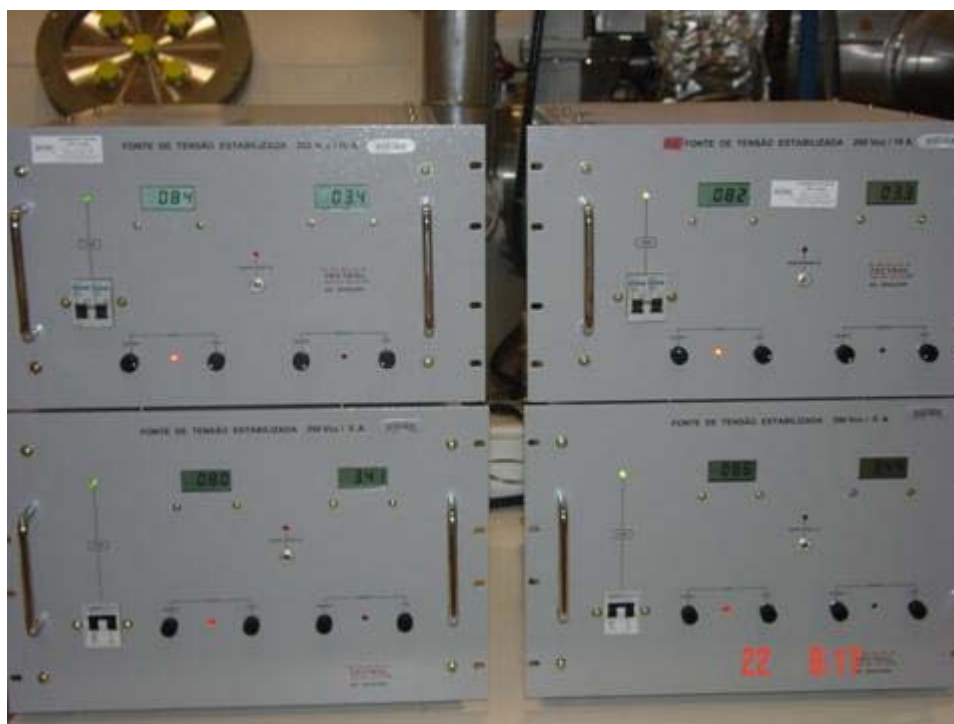
Figure 6: Power supplies (four sources to four lamps).
