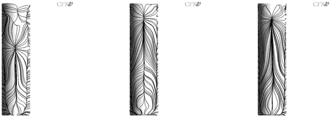
Figure 4: Surface streamlines at rear view of the cylinder - From left to right - URANS, DES and LES
