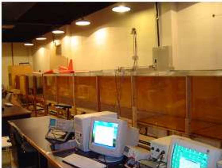
Figure 3: Illustration of the low speed wind tunnel.
