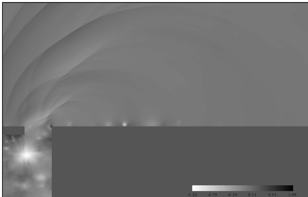
Figure 5. Far-field visualization based on contours of C_p .
