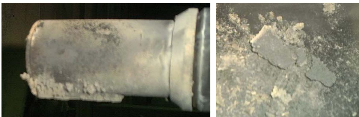
Figure 10 – Photograph of the probe after exposure in the furnace and collected deposits.
