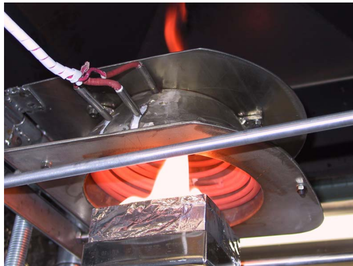
Figure 2 – Burning of a pinus slab in the cone calorimeter.
