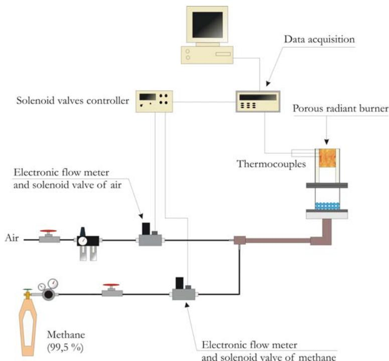
Figure 2. Schematic view the apparatus for testing of radiant porous burners.
