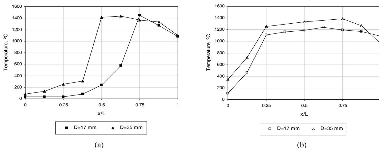
Figure 6. Temperature profiles across the porous burner, for  $\phi = 0,55$ ,  $S_L = 30$  cm/s, with perforated plate of 17 mm and 35 mm, recorded (a) in the central line and (b) in the intermediate line.
