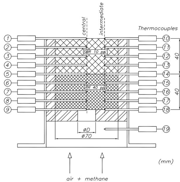
Figure 3. Schematic drawing of the radiant porous burner.
