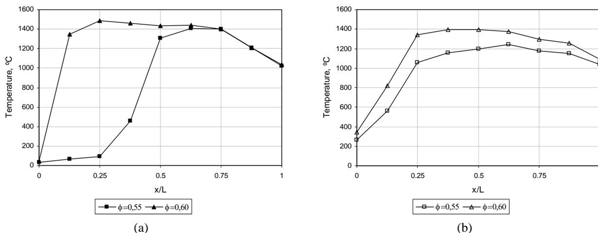
Figure 5. Temperature profiles across the porous burner with a perforated plate of 17 mm, for  $S_L = 30$  cm/s,  $\phi = 0,55$  and  $\phi = 0,60$ , recorded (a) in the central line and (b) in the intermediate line.
