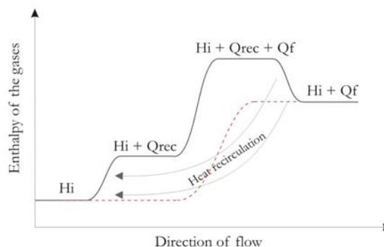
Figure 1. Rendering of the gas and solid enthalpy across a flame within a porous medium, showing the increase of enthalpy in the flame zone as a result of sensible heat recirculation, where  $H_i$  is the initial enthalpy,  $Q_{rec}$  is the recirculated heat and  $Q_f$  is the energy of the fuel (from Hardesty e Weinberg, 1974).
