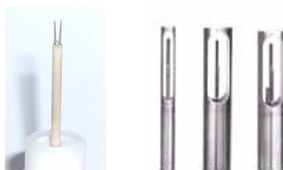
Figure 2. Typical laboratorial (left) and industrial (right) probes of HWA systems.
