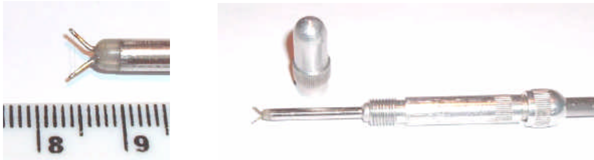
Figure 6. Sensor view. Wire and prongs (at left) and probe body (at right).
