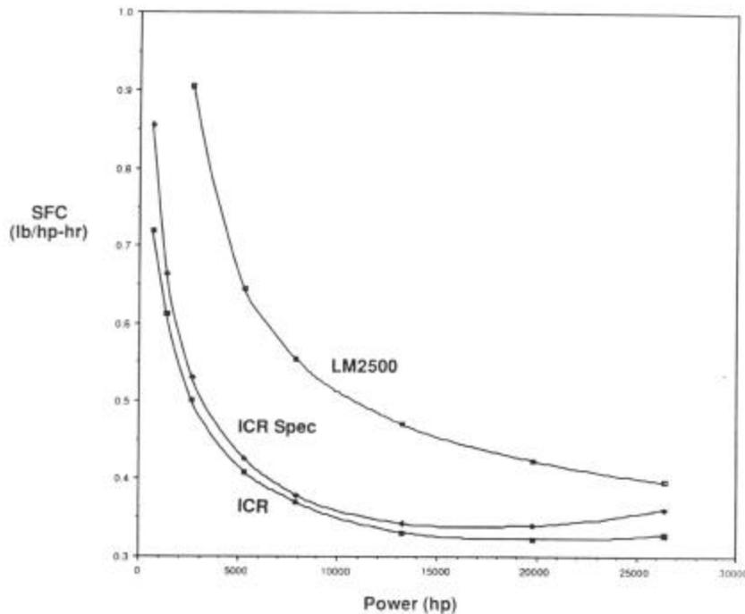
Figure 1 - Performance Comparison of simple and ICR cycles.
