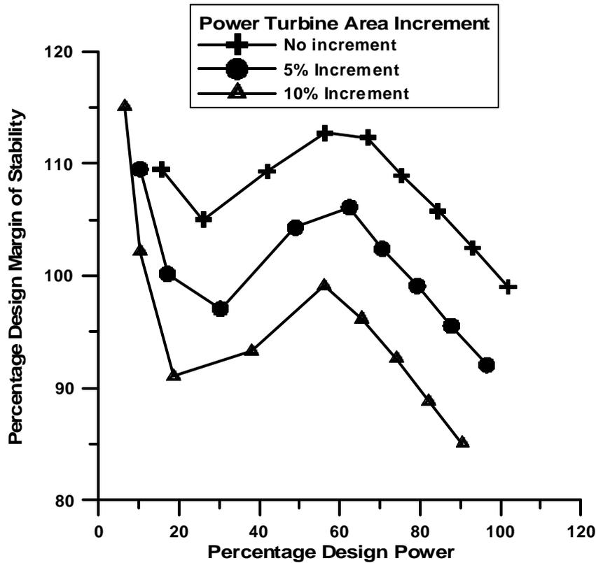
Figure 4 - Surge margin as function of load and NGV setting.
