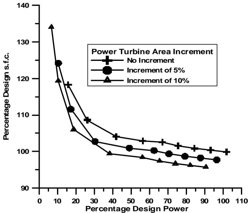
Figure 5 - Specific fuel consumption as function of load and NGV setting.
