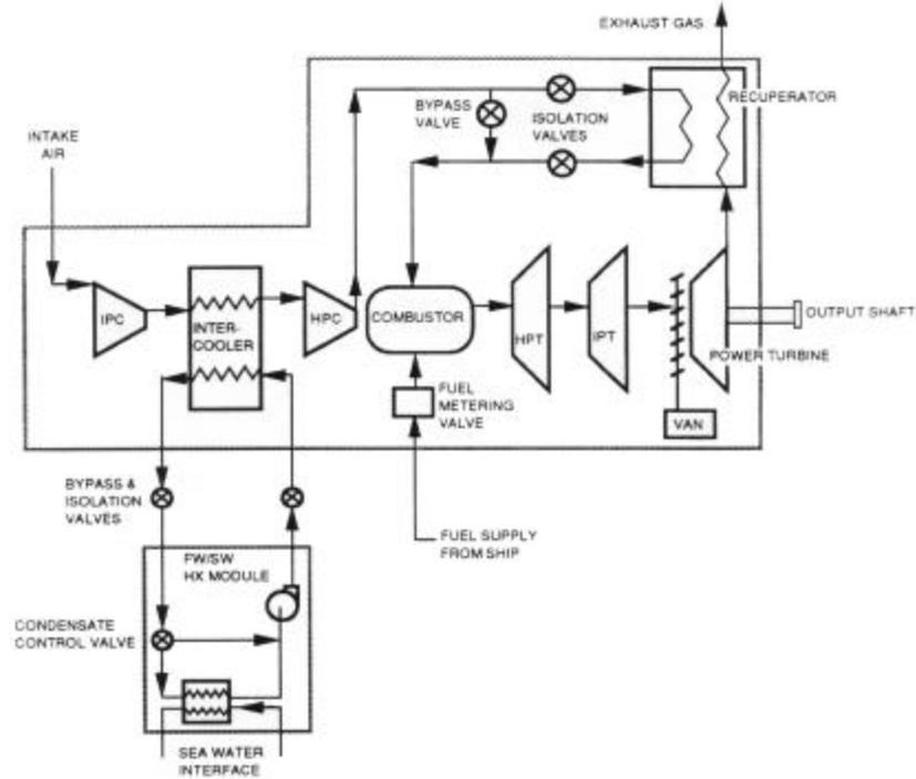
Figure 2 –ICR Functional Operation [12]
