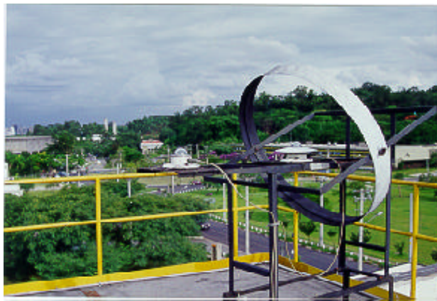
Figure 1a: The IAG site in the University of São Paulo Campus, São Paulo (23° 32'S). The shadow-band device has 40 cm of diameter. The picture reports the Southeast sector of the University Campus, with the Oceanographic Institute behind.
