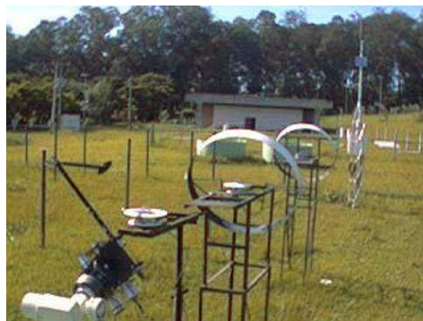
Figure 1b: The UNESP site in the State University of São Paulo, Botucatu, SP (22° 51'S). Both shadow-band devices have 40 cm of diameter. The solar tracker in the up front has a shadow disk coupled in it. The picture reports the Southeast sector the State University of São Paulo campus located at left side of the Department of Environmental Sciences building.
