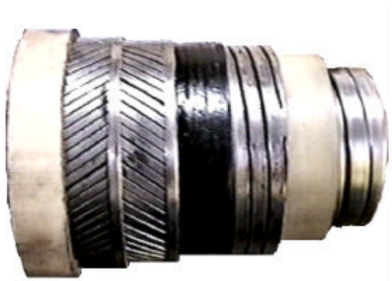
Figure 1 – Typical structure of a subsea flexible line.
