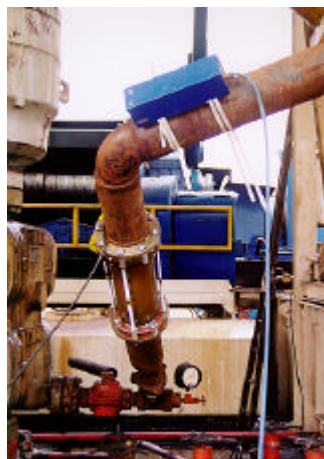
Figure 2 - Relative positions of the acrylic pipe and the SAM 400 sensor.
